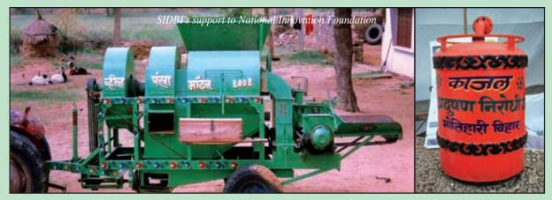
Multi Crop Thresher-machine capable of thrashing all types of crops with minimum changes Used in reducing carbon in the setting of mechanical parts, thus saves time and energy.
