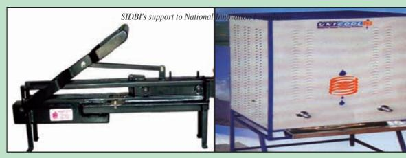
Bamboo Splinter- used for making of splints for agarbatti incense sticks and bamboo mat boards.
