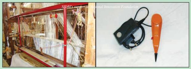
Design making machine- An attachment can be fitted into any handloom Jacquard machine for the insertion of weft threads needed to make a variety of designs.
